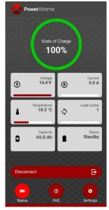
Tip! For the most accurate service report, it is best to create it shortly after the battery is fully charged. The battery is considered sufficiently charged when the voltage displayed in the app is at least 14.4 V.
