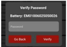
**8.** Enter the battery password. This is required on every device you connect to the battery for the first time. The password can be found on the side of the battery, on the sticker with the serial number, after 'PW'. A card is also included that shows both the serial number and the password.
