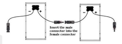
If the mutual distance is too large, you can use the included solar cable to make the connection. The solar cable can be installed into the included cable duct. Perform installation conform the gluing instruction in paragraph 3.5.
