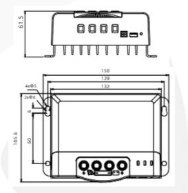
Outline dimensions: 150\*105.6\*61.5mm; Mounting dimensions: 139\*60mm; Fixed holes dia: Φ5mm; Wire specifications: 20-6AWG.
