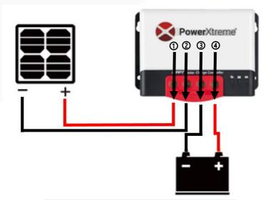
Image 2. Wiring diagram charge controller one solar panel
