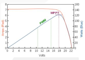
Image 1. Typical output curve solar panel
